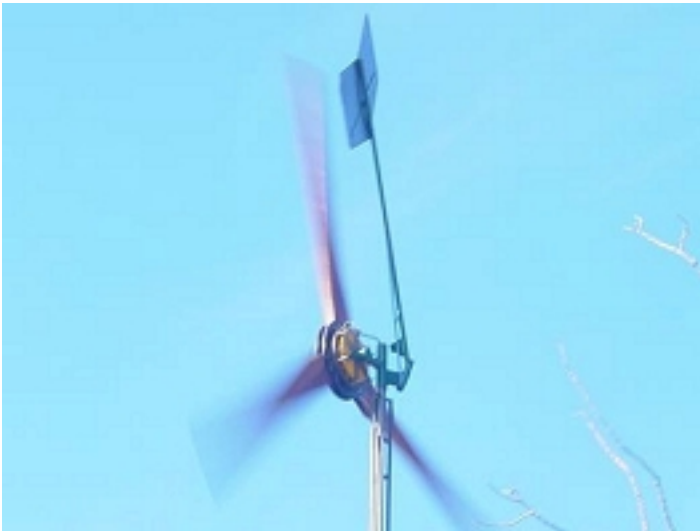
This photo shows a home-built 17-foot diameter 3.5 kW turbine with the tail in fully furlled position. The machine is still making near maximum power, but it facing at an angle into the wind to reduce wind input. Photo by Dan Bartmann.
