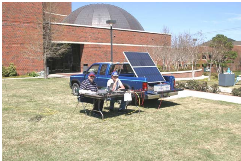
Bill Allen (WA5PB) (l), and Larry D. Barr (K5WLF) at the controls of the Solar Powered Ham Station. In the pickup are the Uni-Solar US 64 amorphous PV panels, Xantrex C12 controller and the PowerSonic PS-121000 100 Ah AGM batteries. The building in the background is the Tarleton State University Science building. The planetarium (Larry's 'real' job) is under the dome.
