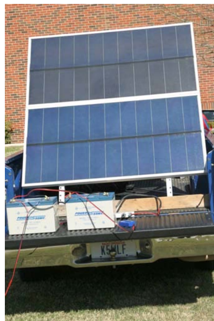
Bill Allen (WA5PB) (l), and Larry D. Barr (K5WLF) at the controls of the Solar Powered Ham Station. In the pickup are the Uni-Solar US 64 amorphous PV panels, Xantrex C12 controller and the PowerSonic PS-121000 100 Ah AGM batteries. The building in the background is the Tarleton State University Science building. The planetarium (Larry's 'real' job) is under the dome.
