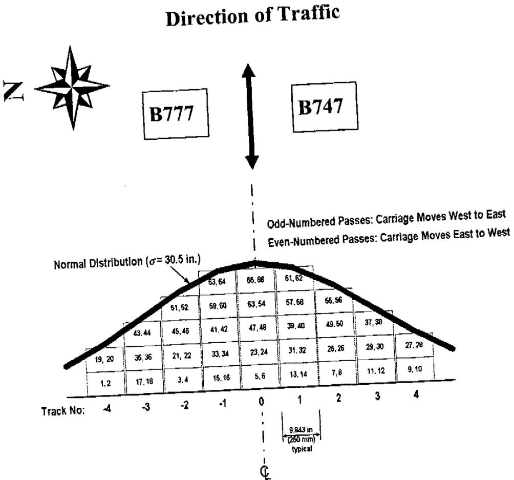
Figure 3. Wander Pattern Used in NAPTF Traffic Testing (Source: <http://www.airporttech.tc.faa.gov/NAPTF/Wander.asp>) (1 in. = 25.4 mm)
