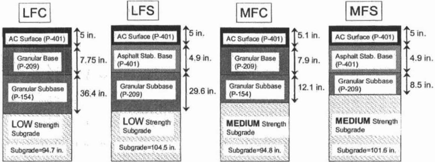
Figure 2. Cross-sectional Views of "As-Built" NAPTF Test Sections (not to scale) (1 in. = 25.4 mm)
