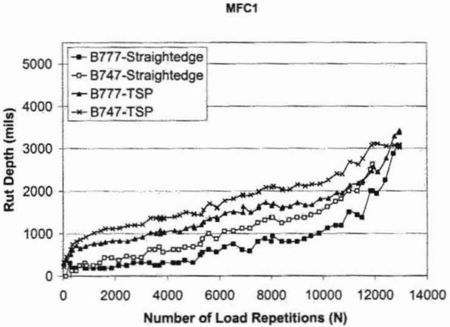
Figure 11. Comparison of Straightedge and TSP Rut Depths for MFC Test Section (1 mil = 0.0254 mm)
