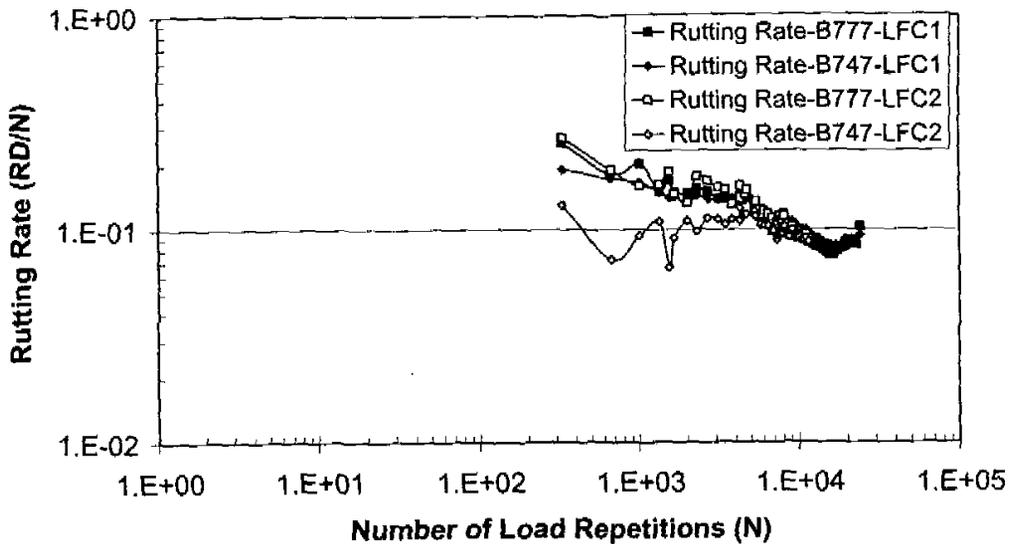
Figure 21. Rutting Rate (RR) Versus Number of Load Repetitions (N) for LFC Sections
