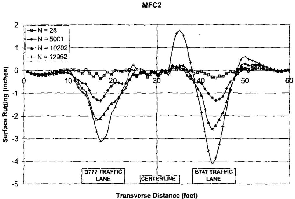
Figure 7. Transverse Surface Profiles (along Profile Lines 1 and 2) at Specific Number of Load Repetitions for NAPTF MFC Test Section (1 ft. = 0.305 m; 1 in. = 25.4 mm)
