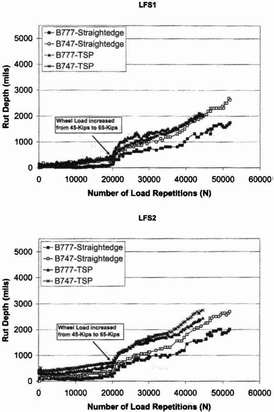
Figure 10. Comparison of Straightedge and TSP Rut Depths for LFS Test Section (1 mil = 0.0254 mm)
