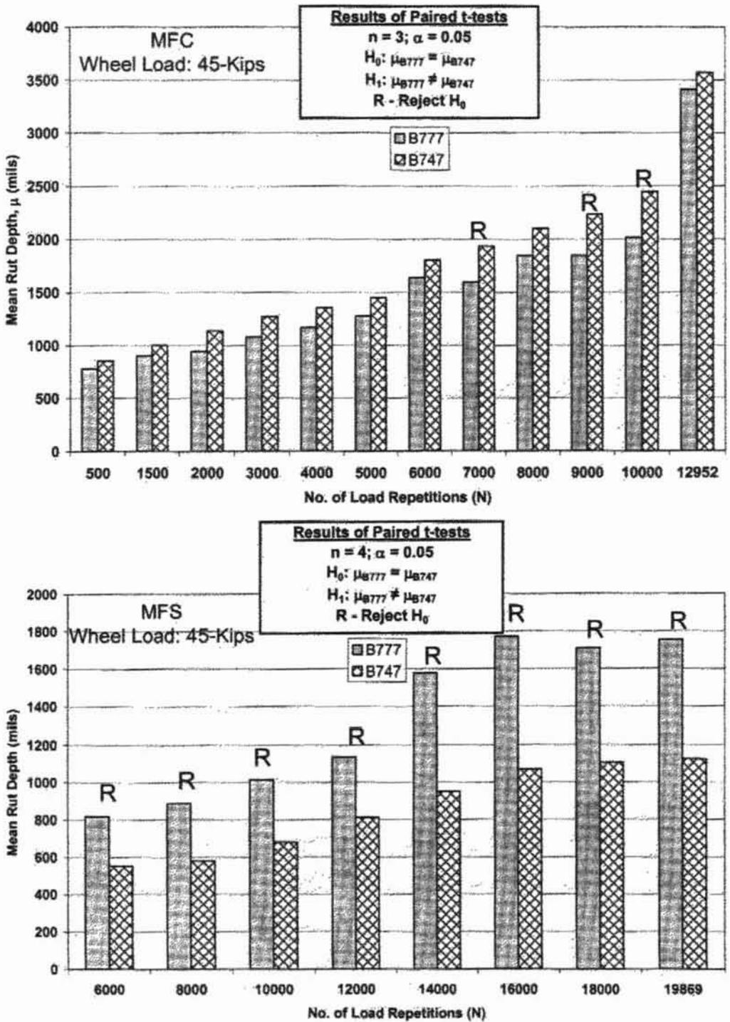
Figure 18. Results of Paired t-Tests between B777 and B747 Mean Rut Depths for Medium-Strength Test Sections (1 Kip = 0.45 tonnes; 1 mil = 0.0254 mm)
