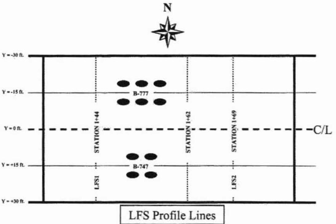
Figure 13. Location of Profile Lines for TSP Measurements in Low-Strength Test Sections (1 ft. = 0.305 m)
