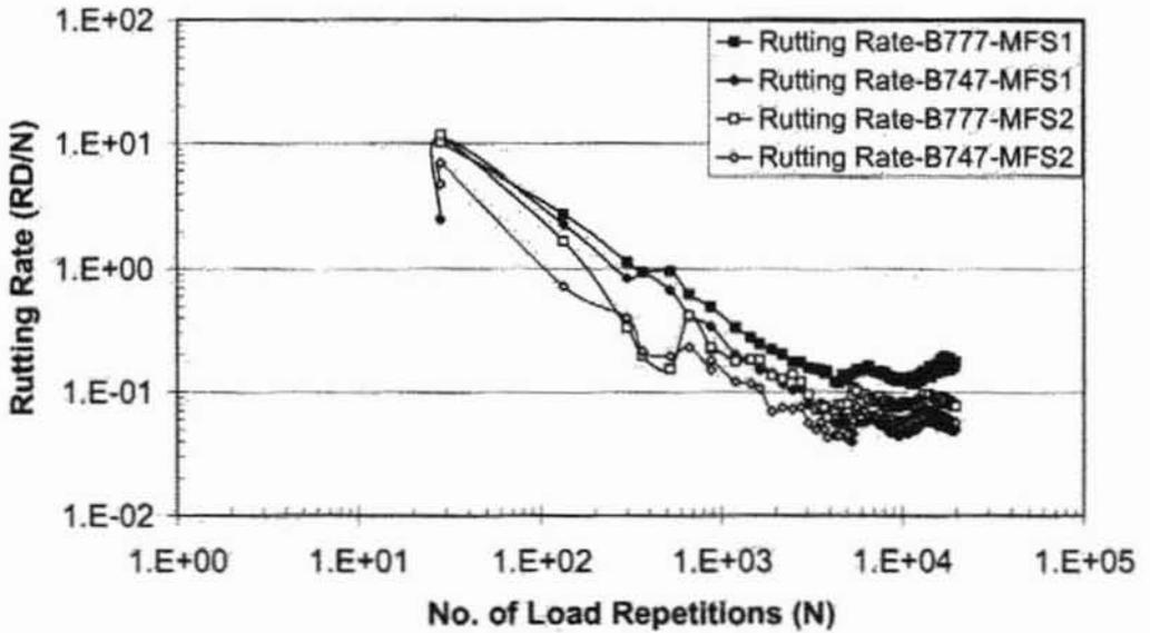
**Figure 23. Rutting Rate (RR) Versus Number of Load Repetitions (N) for Medium-Strength Sections (1 Kip = 0.45 tonnes)**
