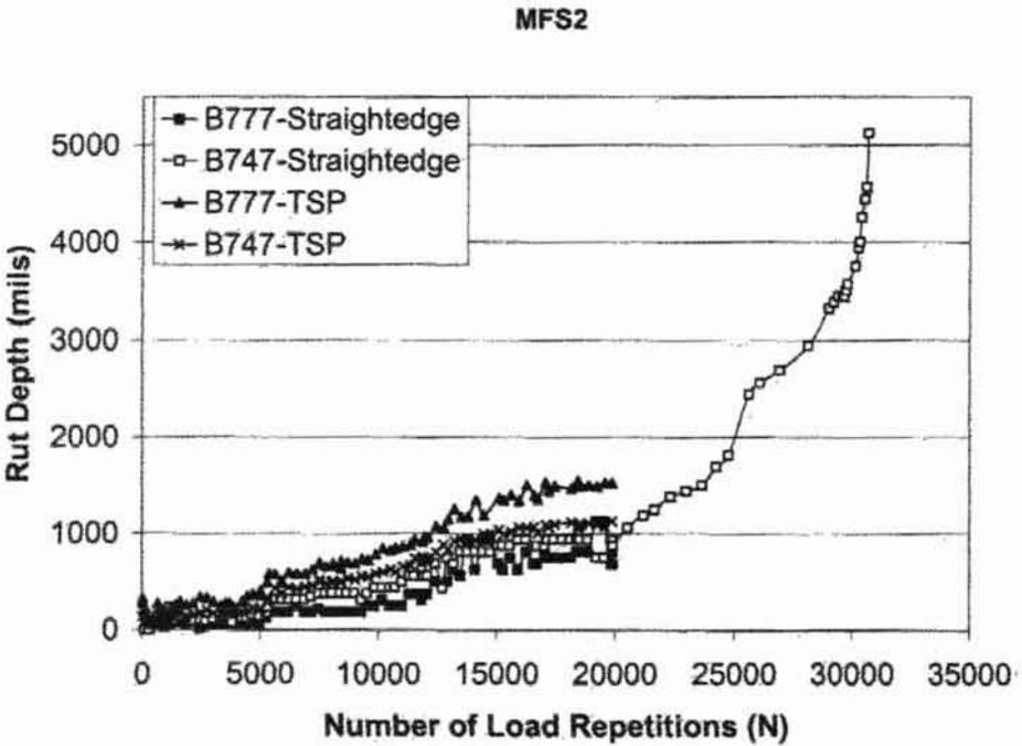
**Figure 12. Comparison of Straightedge and TSP Rut Depths for MFS Test Section (1 mil = 0.0254 mm)**
