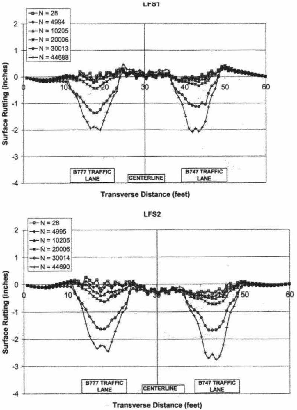
Figure 6. Transverse Surface Profiles (along Profile Lines 1 and 2) at Specific Number of Load Repetitions for NAPTF LFS Test Section (1 ft. = 0.305 m; 1 in. = 25.4 mm)
