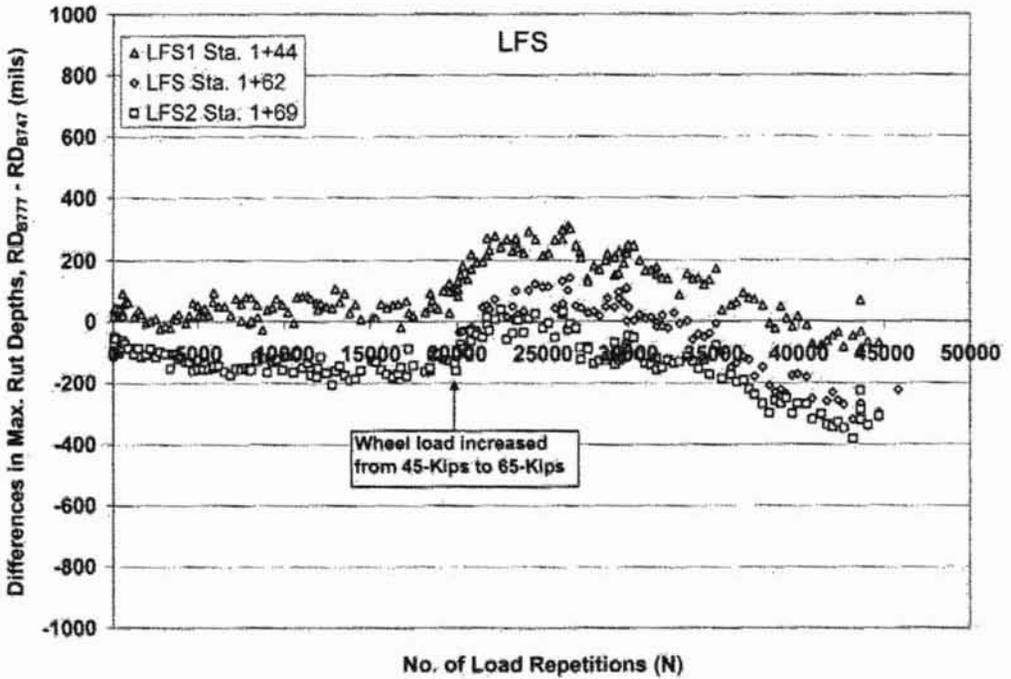
Figure 15. Differences in Maximum Rut Depths between B777 and B747 Trafficking for Low-Strength Test Sections (1 Kip = 0.45 tonnes; 1 mil = 0.0254 mm)
