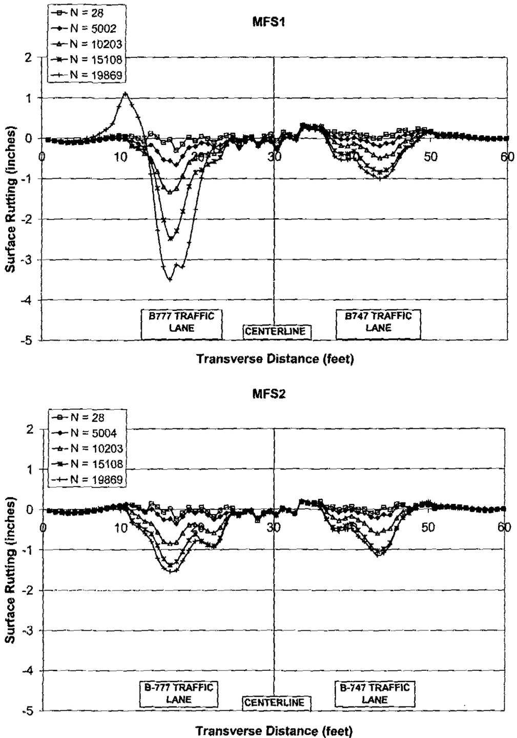
Figure 8. Transverse Surface Profiles (along Profile Lines 1 and 2) at Specific Number of Load Repetitions for NAPTF MFS Test Section (1 ft. = 0.305 m; 1 in. = 25.4 mm)
