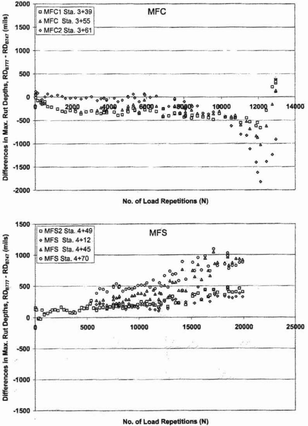
Figure 16. Differences in Maximum Rut Depths between B777 and B747 Trafficking for Medium-Strength Test Sections (1 Kip = 0.45 tonnes; 1 mil = 0.0254 mm)
