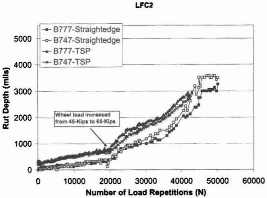
**Figure 9. Comparison of Straightedge and TSP Rut Depths for LFC Test Section (1 mil = 0.0254 mm)**
