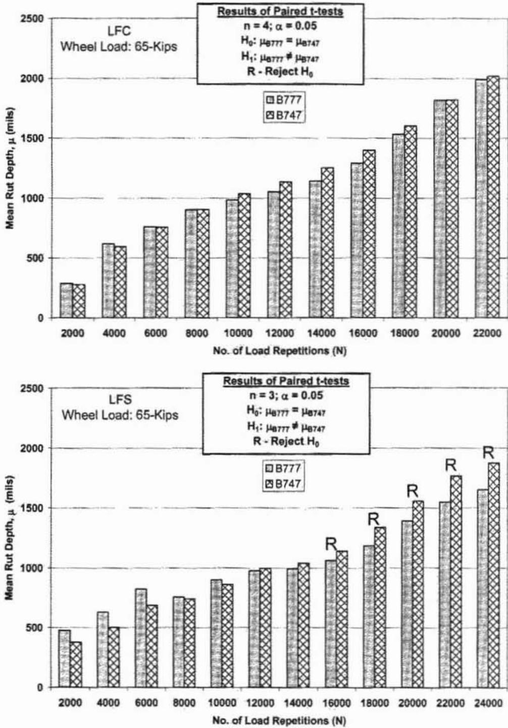
Figure 17. Results of Paired t-Tests between B777 and B747 Mean Rut Depths for Low-Strength Sections (1 Kip = 0.45 tonnes; 1 mil = 0.0254 mm)
