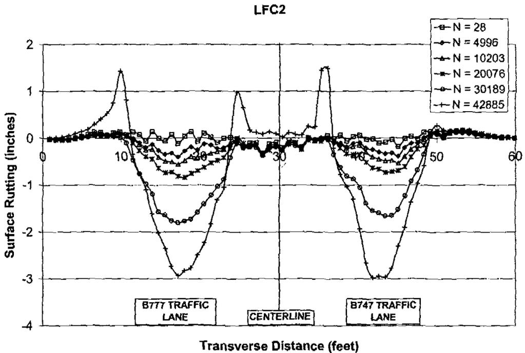
Figure 5. Transverse Surface Profiles (along Profile Lines 1 and 2) at Specific Number of Load Repetitions for NAPTF LFC Test Section (1 ft. = 0.305 m; 1 in. = 25.4 mm)
