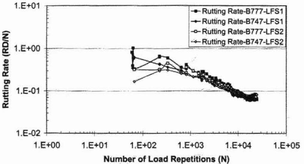
**Figure 22. Rutting Rate (RR) Versus Number of Load Repetitions (N) for LFS Sections (1 Kip = 0.45 tonnes)**
