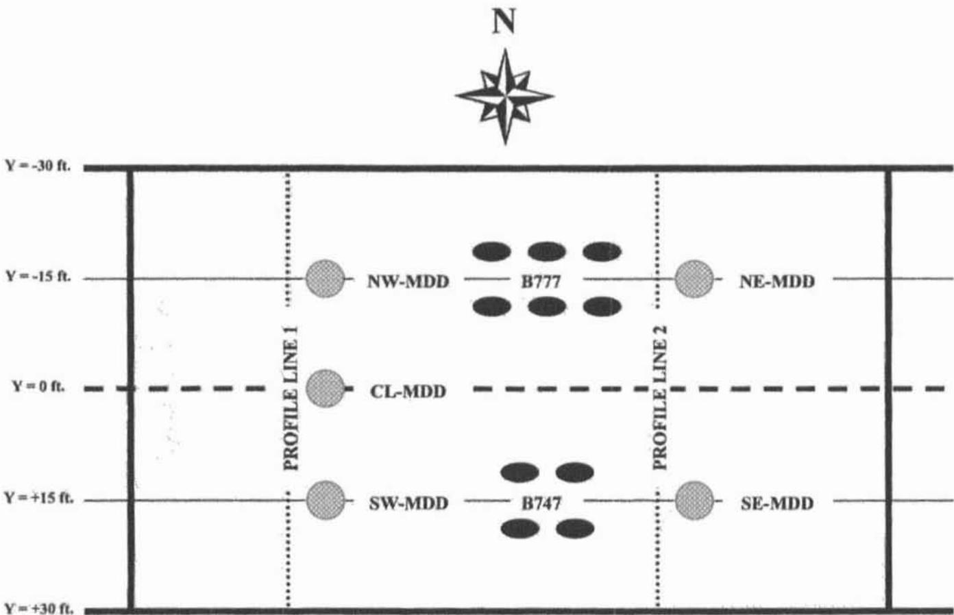
Figure 4. Location of Main Profile Lines in NAPTF Flexible Test Items with Respect to MDD Instrumentation (1 ft. = 0.305 m)
