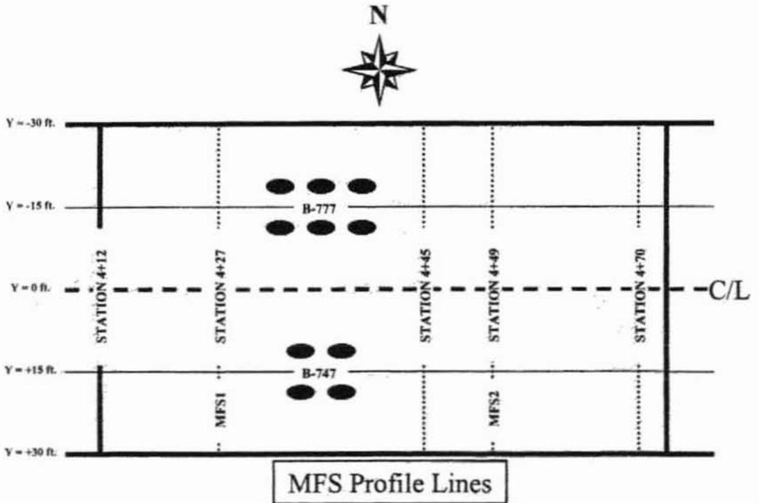
Figure 14. Location of Profile Lines for TSP Measurements in Medium-Strength Test Sections (1 ft. = 0.305 m)
