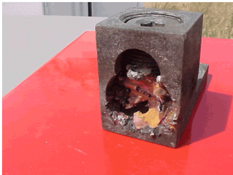
Figure K-2. Destroyed Mechanical Terminal From PV System
