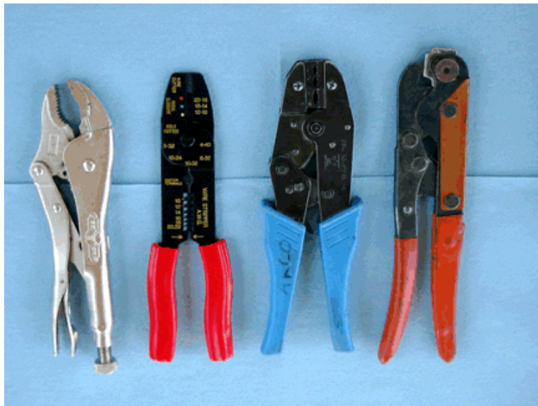
Figure 4. Terminal Crimping Tools-Two on Left Unlisted, Two on Right Listed
