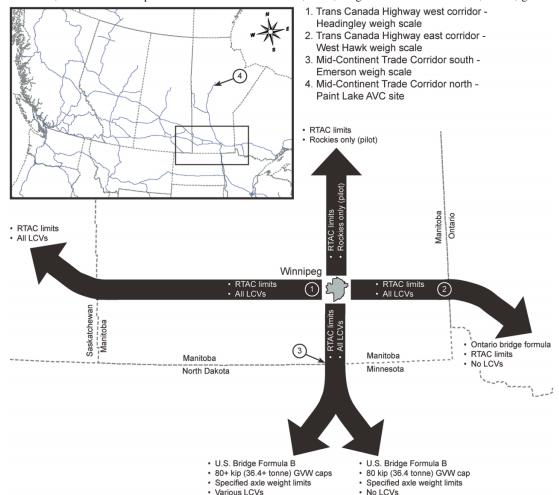
Fig. 1. Schematic of fleet mix analysis network in relation to the Canadian National Highway System network and U.S. Interstate Highway System network. RTAC, Roads and Transportation Association of Canada; LCV, longer combination vehicles; GVW, gross vehicle weight.
