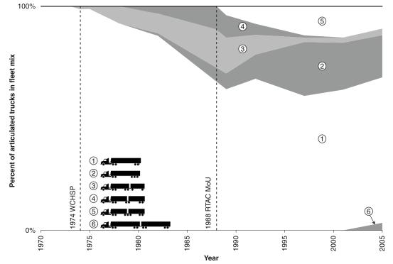
Fig. 2. Articulated truck fleet mix on the Trans Canada Highway west corridor. WCHSP, Western Canada Highway Strengthening Program; RTAC MoU, Roads and Transportation Association of Canada Memorandum of Understanding on Heavy Vehicle Weights and Dimensions.
